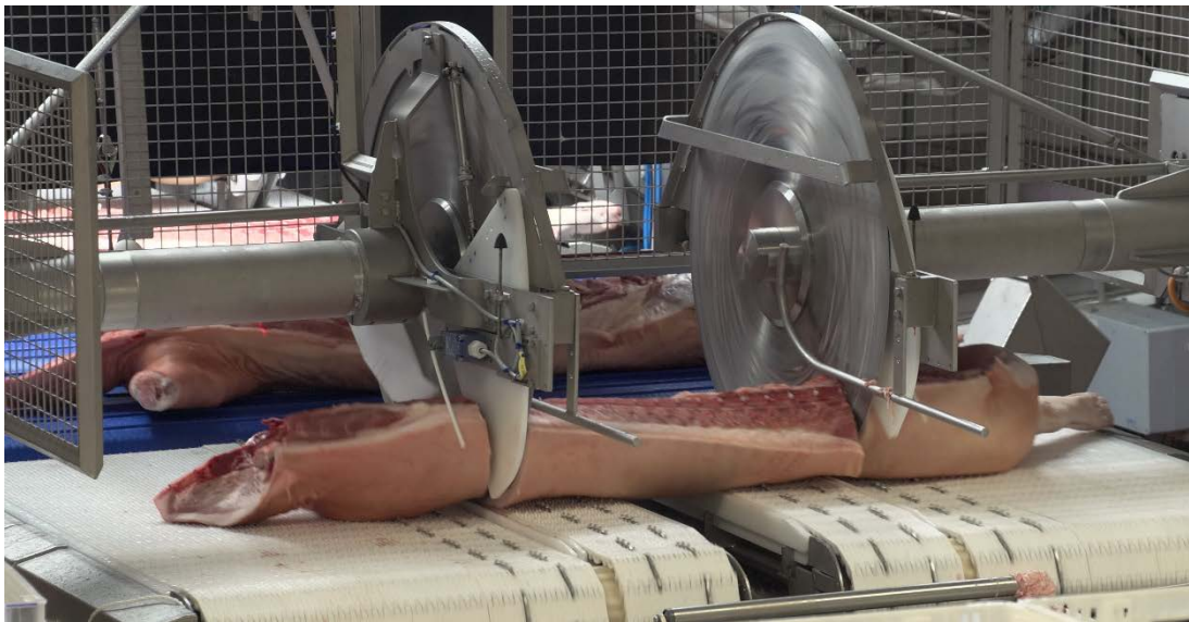
Figure 7 Laser-driven cutting positioning for dividing carcasses. Photo courtesy of Marel Red Meat Slaughtering
