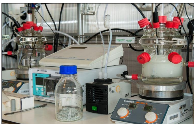
Experimental set-up to study bio-crystallization of metals
