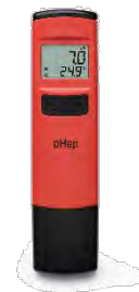
Figure 6. pH pocket meter
