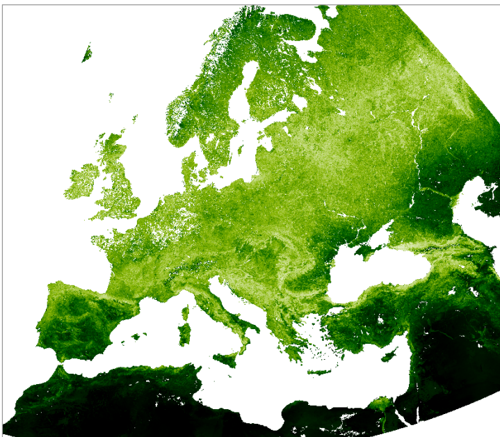
Figure 1. Example of SPOT NDVI decade data for Europe (Light green: high NDVI; dark green: low NDVI; white: water/no data). Third 10 day-period in June 2007.
