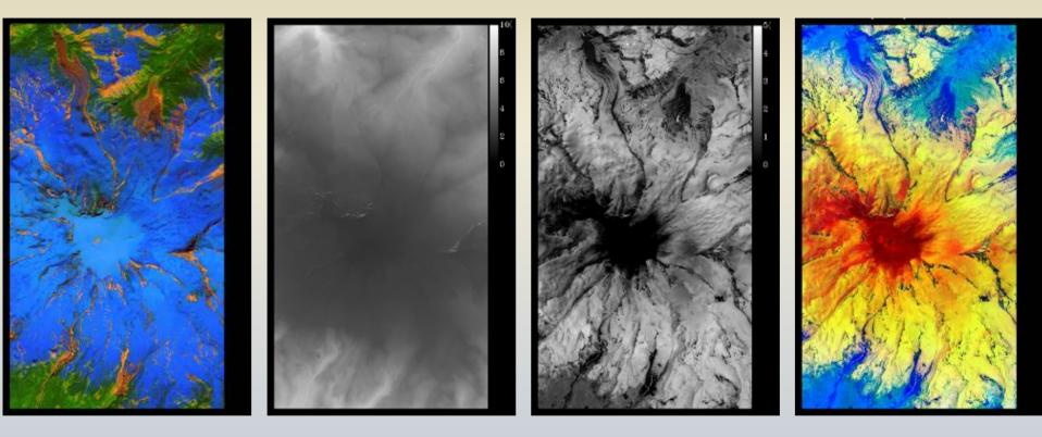
AVIRIS image, 409, 1324, 2269 nm precipitable water, I-8 mm liquid water, 0-5 mm path absorption vapor, liquid, ice (BGR)
