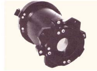
Fig. 5. VNIR spectrometer assembly.
