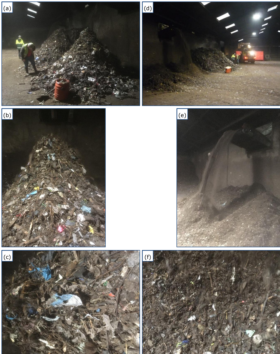
Figure 14 Fractions collected after the first composting and sieving cycle Left: Fraction 3 (>40 mm); (a) sampling under the conveyer belt, (b) close up, (c) further close up. Right: Fraction 5 (10-40 mm); (d) sampling under the conveyer belt, (e) close up, (f) further close up.
