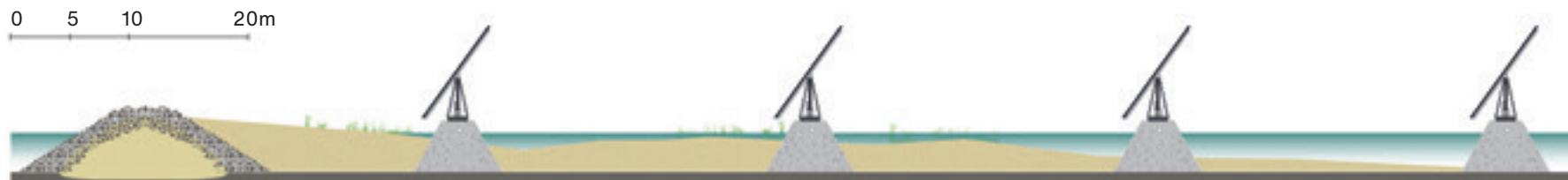
Figure 6.9: Section of the breakwater in combination with the eco-concrete foundations of the solar along a sandy gradient
