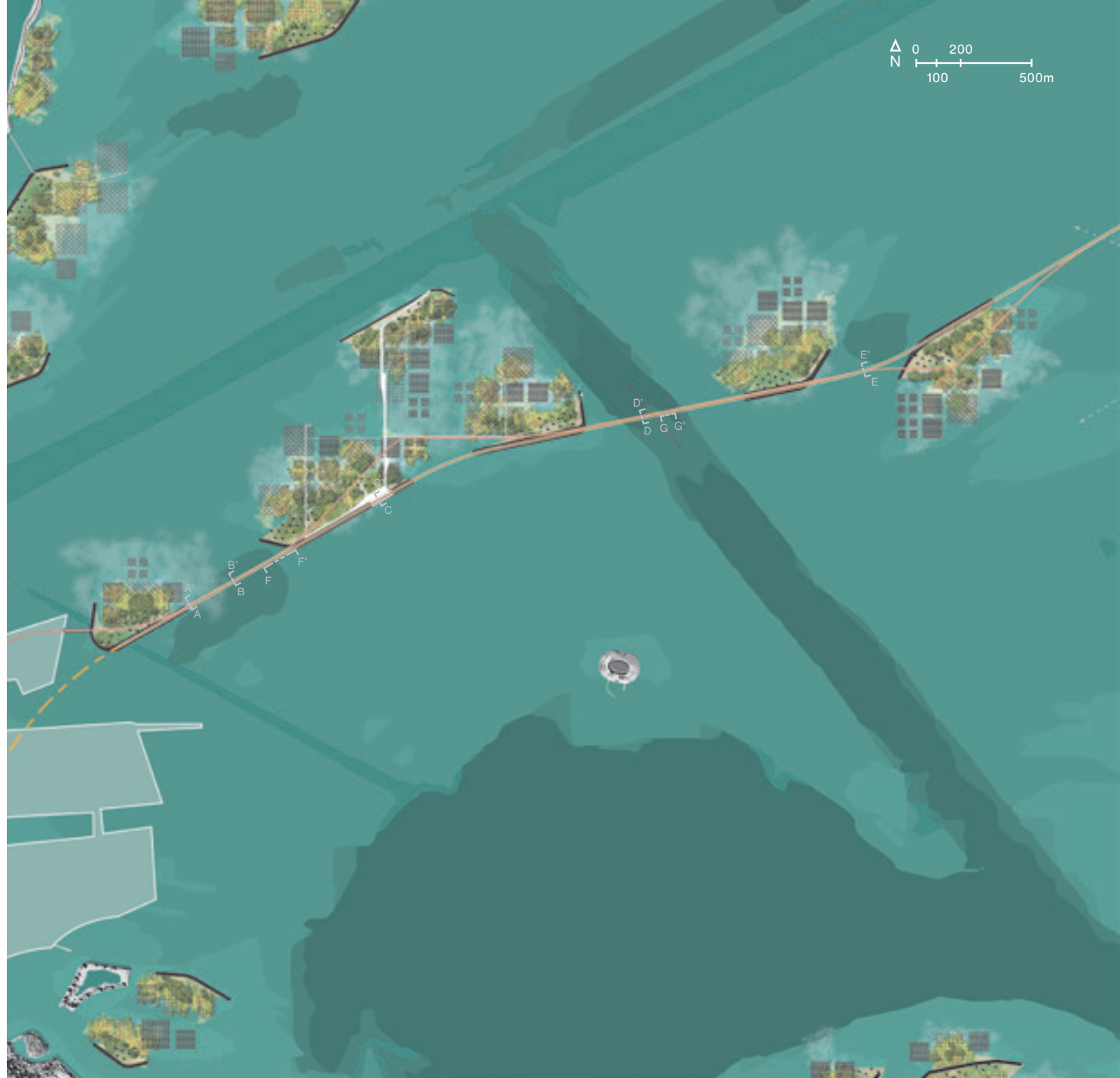
Figure 7.7: Plan of a situation of the Pampus causeway, later in the implementation and succession process. The breakwaters provide a foundation for a railway and bicycle bridge
