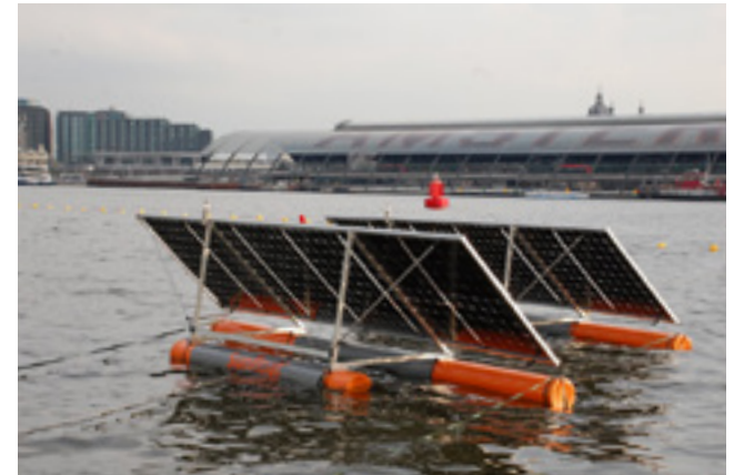
Figure 5.8: Pilot study with floating bifacial PV systems in the IJ in Amsterdam
