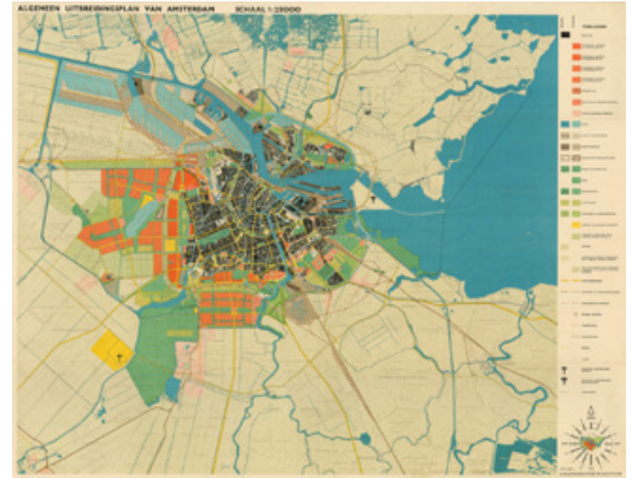
Figure 4.5: The expansion plan of Amsterdam (AUP) of 1934 by van Eesteren, predetermining the green 'wedges' of Amsterdam
