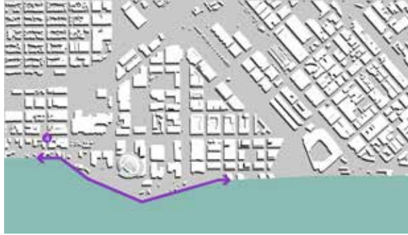
Bay Shoreline Concept 1 is a straightforward earthen levee proposal along the existing waterfront
