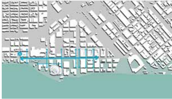
Bay Shoreline Concept 3 positions water protection at 3rd street as it is elevated and converted to the primary line of defense as a dike
