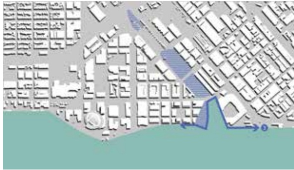
Creek Concept 3 builds levee and wetland protection at the creek's mouth at China Basin; the remaining channel would become a freshwater runoff impoundment.
