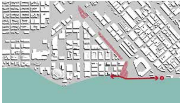
Creek Concept 2 places a tidal control line outside of China Basin; it would also require transitions to elevated adjacent parkland as well as modifications to the stormwater pump station at the end of the Mission Creek channel
