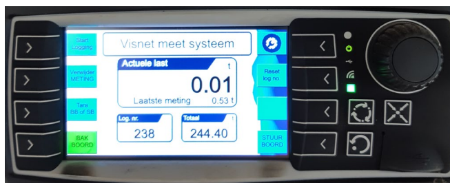
Figure 2: Console with pre selection "portside" before weighing. Photo: Tom Bangma
