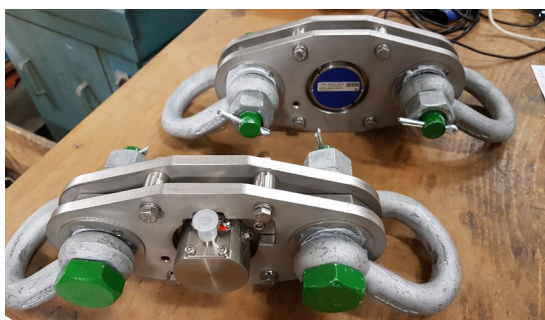
Figure 3: Load cells with safety plates. Photo: Pat Kruger
