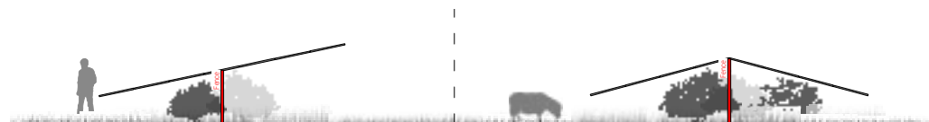
Figure 8.5.2.1: Additional fence running parallel to array
