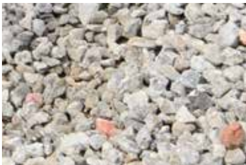
Figure 8.4.5.6: Gravel made of shredded concrete
