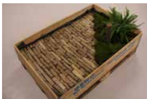
Figure 8.4.5.10 Mock-up stretcher bond parcel direction
