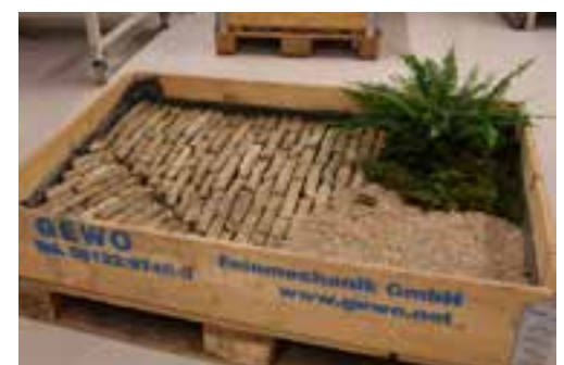
Figure 8.4.5.14: Mock-up polder pattern combined with gravel
