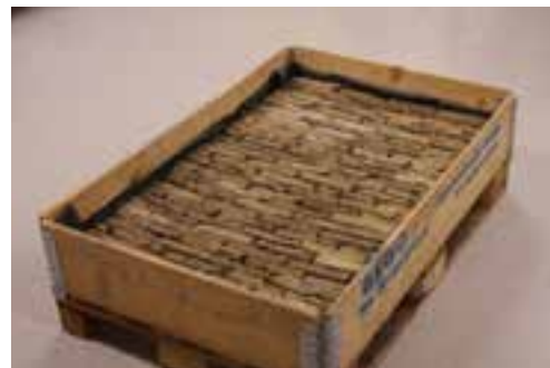
Figure 8.4.5.7: Mock-up stretcher bond
