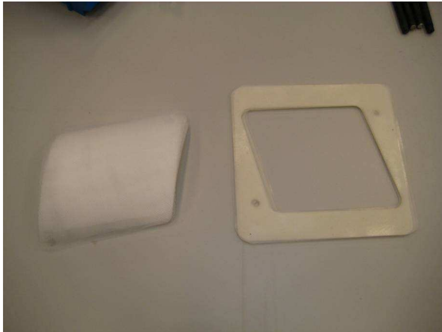
Links: Spacers Rechts: Siliconen pakking
