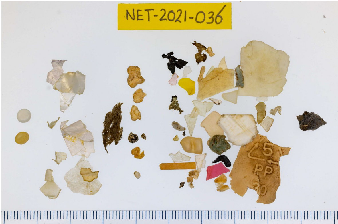
Photo 2. Easy polymer identification in fulmar stomach contents. Sometimes the plastic particles found in fulmar stomachs reveal their polymer composition without further analysis. In this case, a second-year female fulmar, found by Jan van Franeker and Yvonne Hermes on Texel in 2021, contained a plastic fragment labelled as 'PP' – polypropylene. Usually a more complex procedure is necessary to identify the polymer type. In 2021, Kühn et al. (2021b) published a paper where plastic items, ingested by fulmar from the Netherlands, the Faroe Islands and Svalbard were compared: most items were made of polyethylene and polypropylene, reflecting the globally most commonly produced plastic types.
