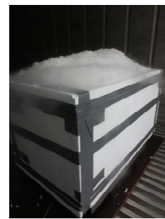
Example of dry ice as a source of CO 2 .
