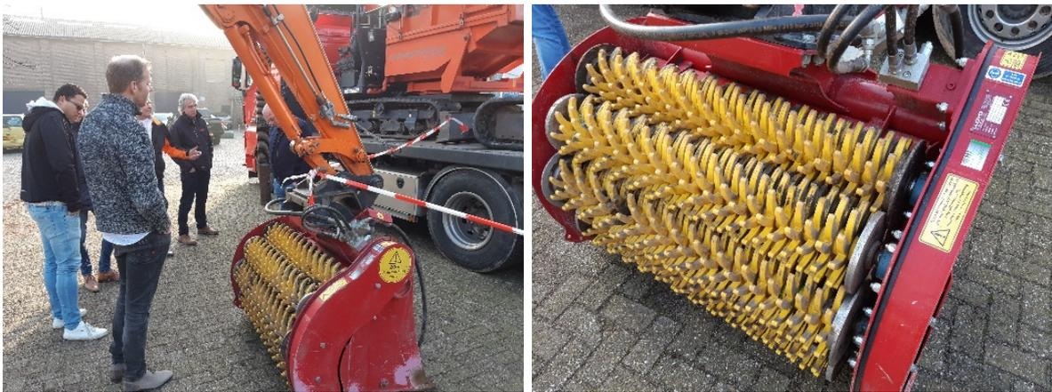
**Figure 9** Mobile crane with bucket and rotating 'fingers' for digging and sifting. The soil falls through the bucket while larger segments (>2 cm) remain inside.
