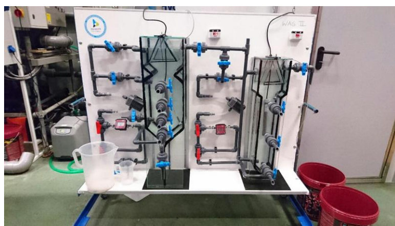
Figure 1. An empty self-constructed anaerobic reactor set comprising an upflow anaerobic sludge blanket (UASB) reactor, and an expanded granular sludge blanket (EGSB) reactor
