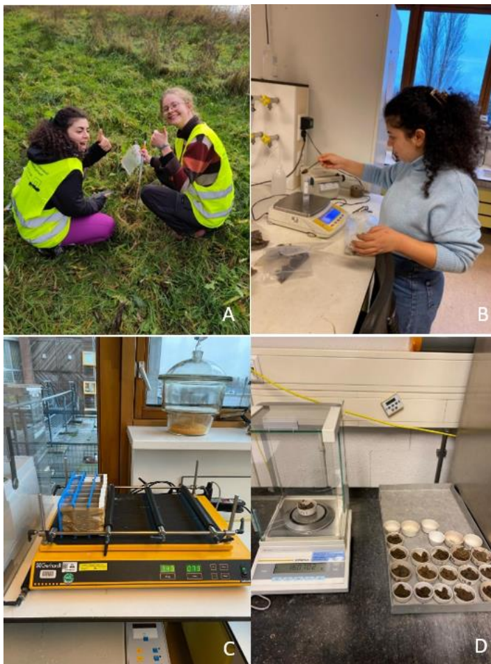
Figure 13. A: Soil sampling with gouge auger on the estate. B: Measuring soil sample to centrifuge tubes. C: Put soil samples to mechanical shaker to equilibrate the samples. D: Weighing samples before drying in the oven.
