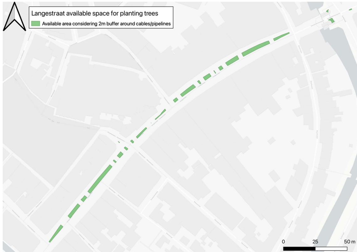
Figure J.1 - The available space for the planting of trees considering a buffer of 2 meter around the cables and pipelines.
