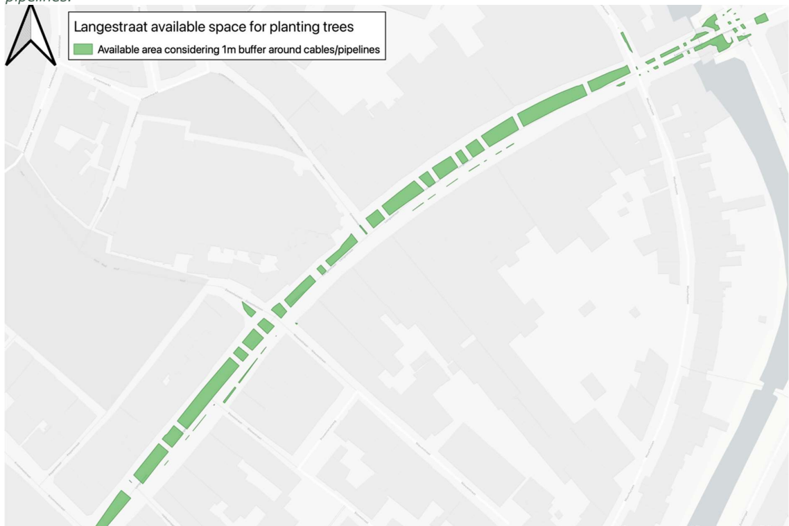
Figure J.2 - The available space for the planting of trees considering a buffer of 1 meter around the cables and pipelines.
