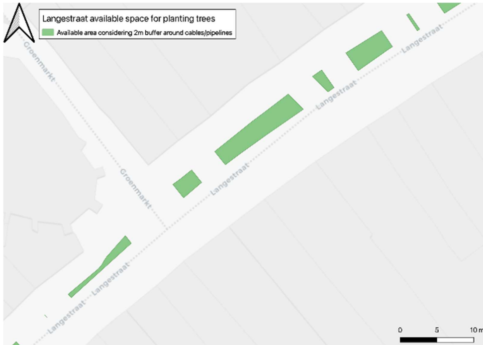
Figure 32 - The available space for the planting of trees considering a buffer of 2 meters around the cables and pipelines
