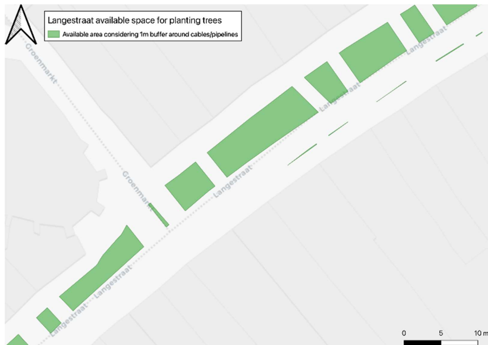
Figure 31 - The available space for the planting of trees considering a buffer of 1 meter around the cables and pipelines.
