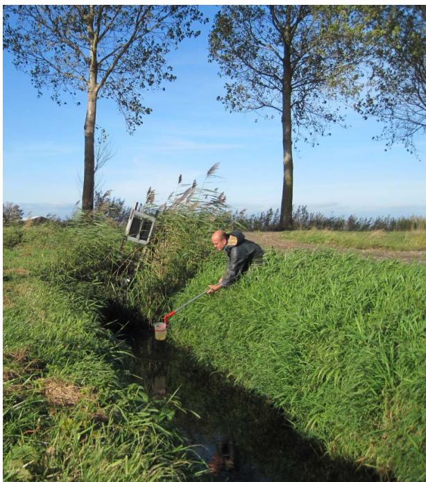
Figure 3.4 Sampling of ditch water using a jug
