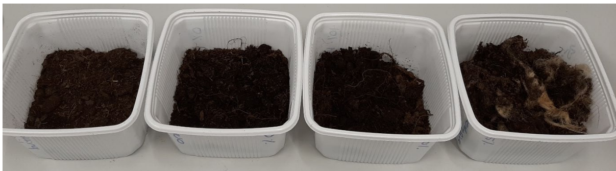
Figure 5. Photographs of the soil containing samples after drying in a vacuum oven overnight. From left to right: potting soil, 0% wool, 10% wool, and 25% wool.
