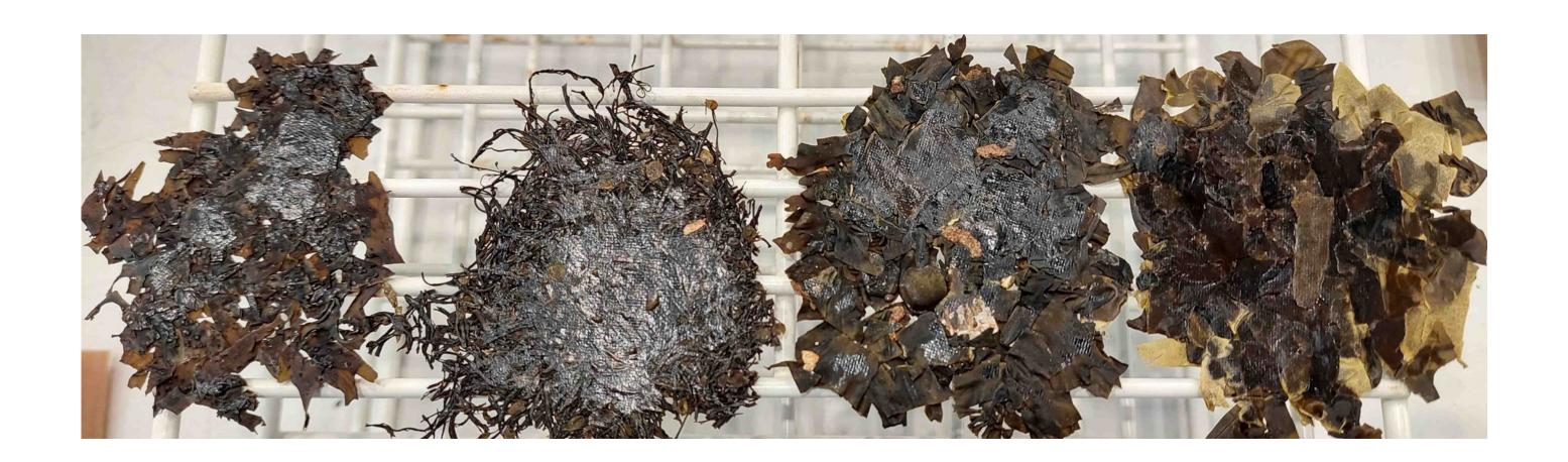
In a follow up, seaweed was pretreated and mixed with reed as a fiber source, aiming to move properties towards conventional particle board materials (picture right).
