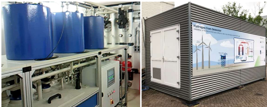
Figure 3: Membrane distillation system (left) in transportable lab with Visual of the project on the outside wall (right).
