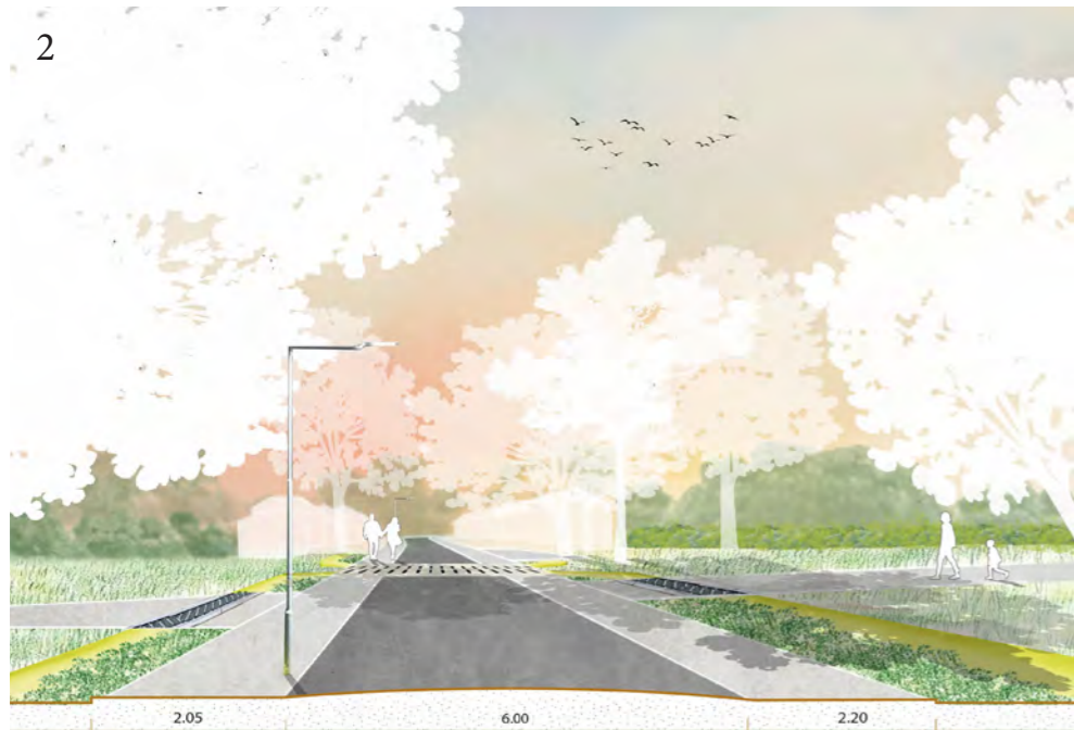
2 Visual water side regulated street; it eliminates the need for curbs and drainage pits, which pose as barriers in the landscape for amphibians. The road is slightly sloped higher toward the middle, rainwater will flow towards the lowest point, into the green area next to the sidewalk
