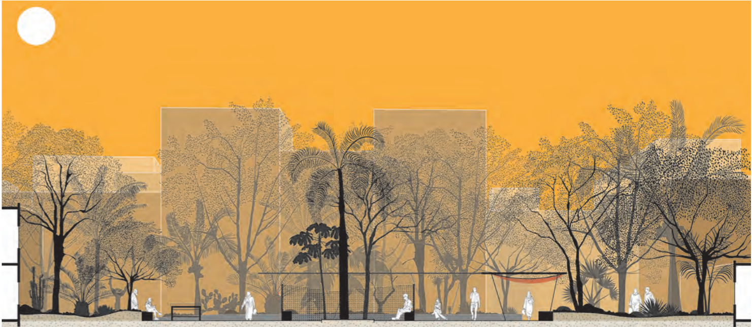
Section of site-design, illustrating the planting beds with varying vegetation, evaporative wall, and louvres with canvas canopies.
