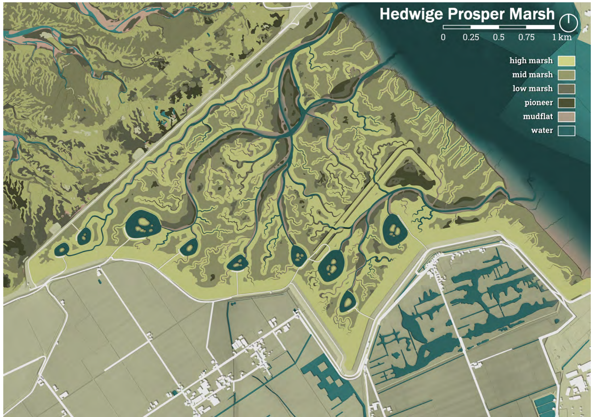
Masterplan: the Hedwige Prosper Marsh. It mostly resembles a natural marsh. An important difference is the high foreshore seawards of the dyke to improve coastal defense. The high foreshore keeps up with sea level rise by sediment supplies cyclically (ca. every twenty years) excavated from several pits. Within these pits, bird islands are present.
