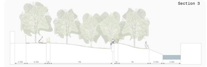
Sections of the Herman Moerkerkplein show different elevation heights and principles of bio-climatic design applied at the design, such as increase of vegetation and a variety of vegetation heights.. In these sections it is clearly shown how the old structure of the city wall is revealed by using vegetation and elevation.
