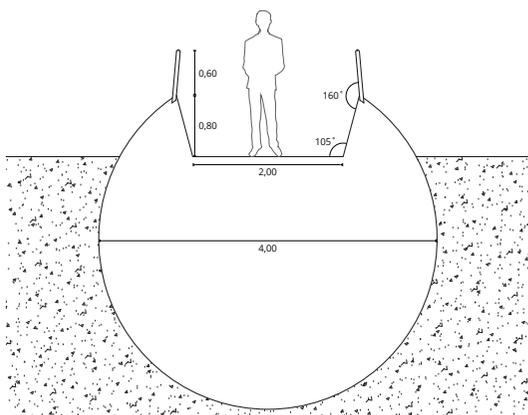
Section of the path cut from the turbine tower (m)
