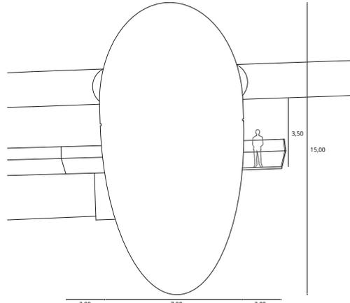
Section of the turbine nacelle and surrounding platform (m)
