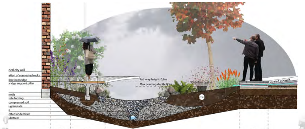
Cross-section of rain garden De Vestingtoren during clear weather or moderate rainfall
