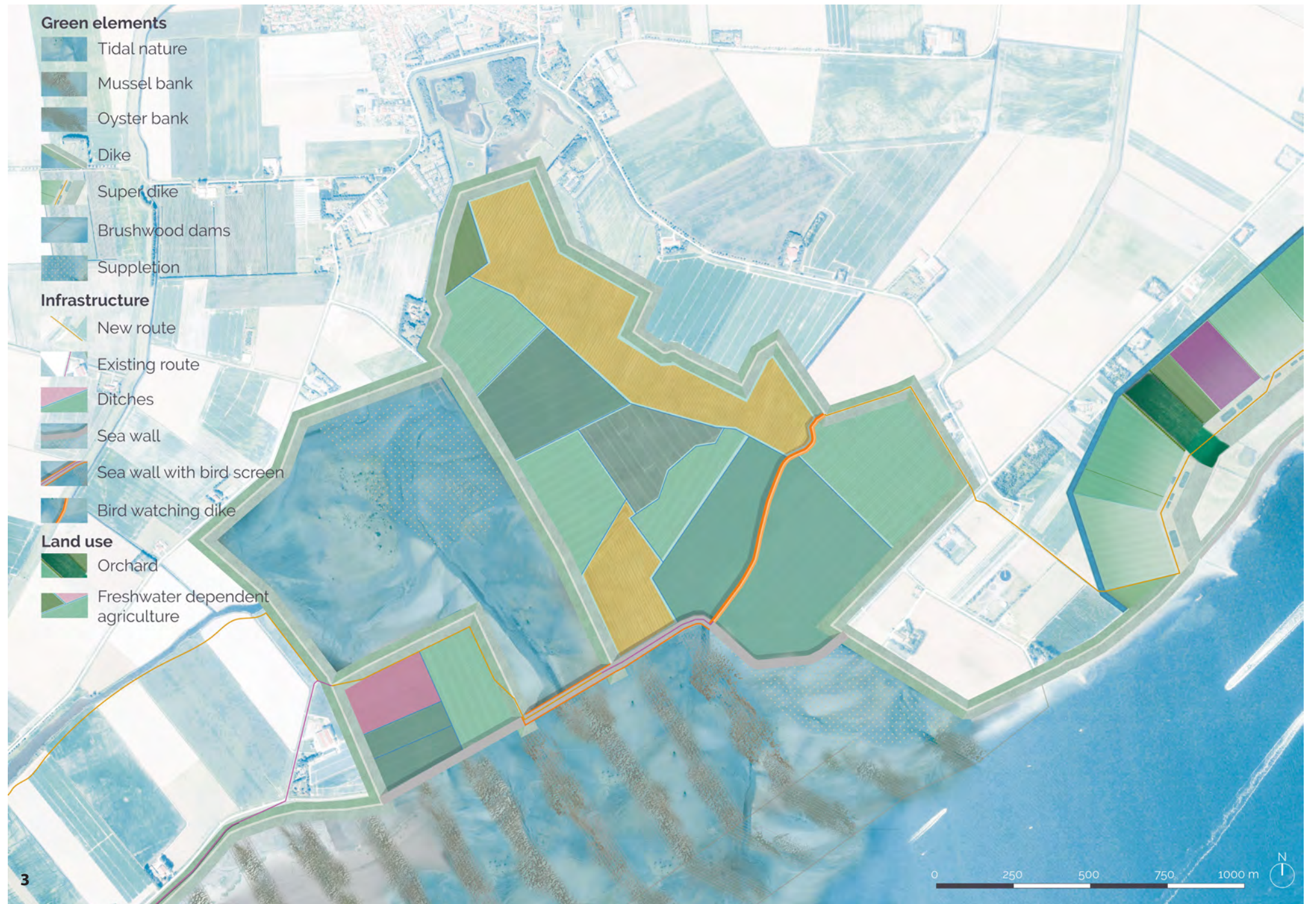
The final detailed design in three steps. A switching landscape to let problematic land silt up with SLR for nature and agriculture on the long term, with an open Oosterschelde barrier.
