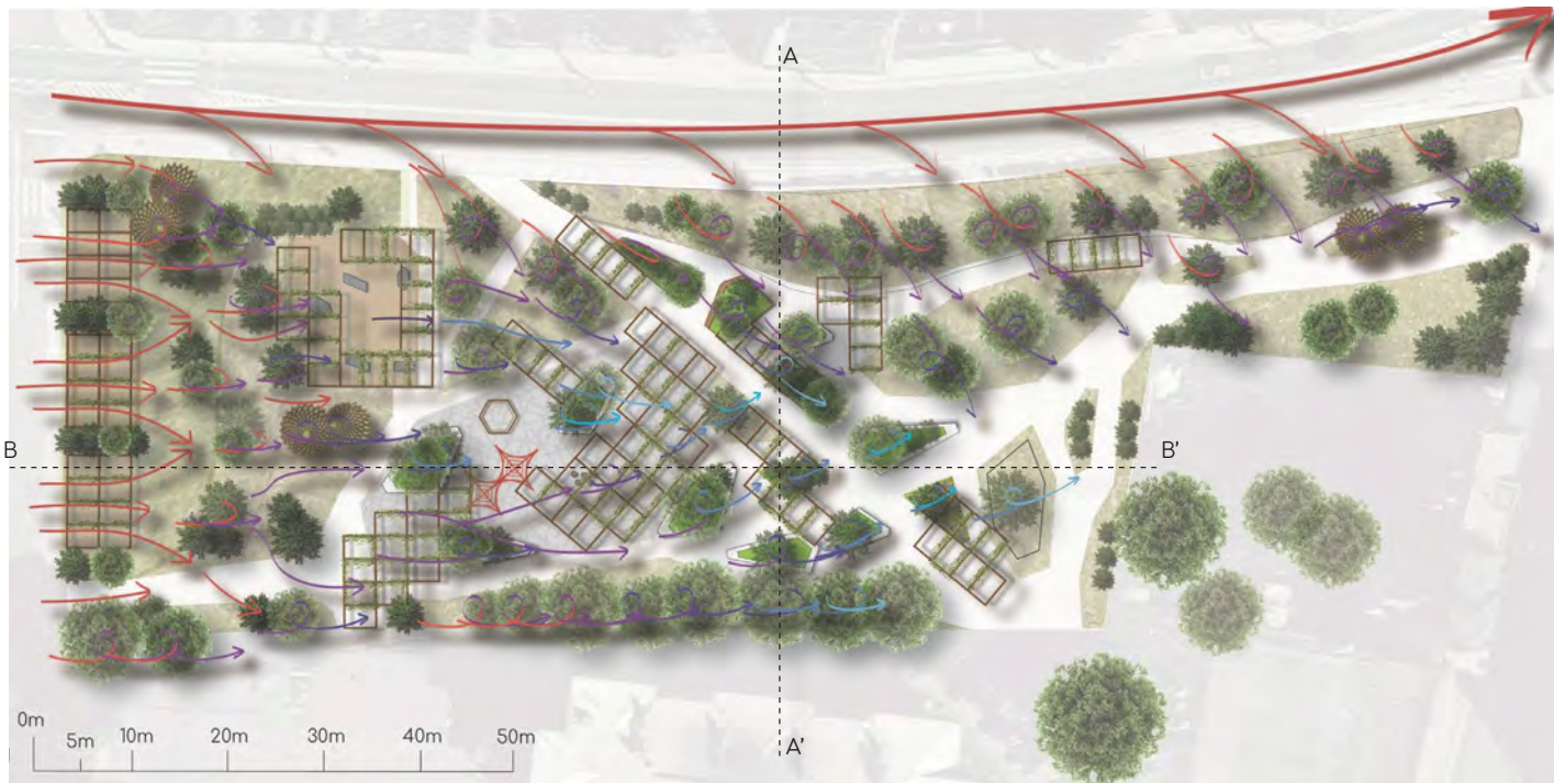
Site design with filtering mechanism in case of predominant west wind direction
