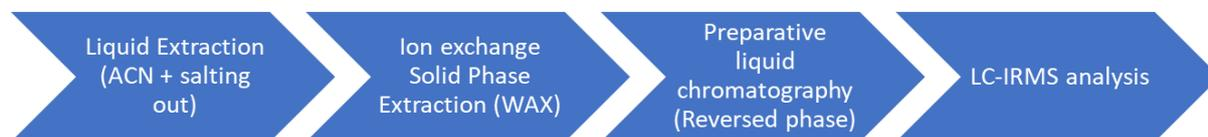
**Figure 3.3** Schematic overview of the developed clean-up for 2-thiouracil in bovine urine samples.
