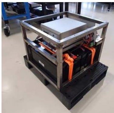
Figure 3 Sensor for, among other things, sensing of Ethylene manufactured by EMS, so-called SKID (source: EMS)
