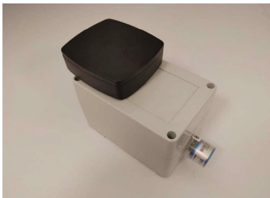
Figure 13 In house developed Printed Circuit Board (LxWxH = 157x80x100 cm., 250 gram) for detecting ethylene gasses in closed environments and determining location based on various GPS satellites (Source: Impact Smart Solution)
