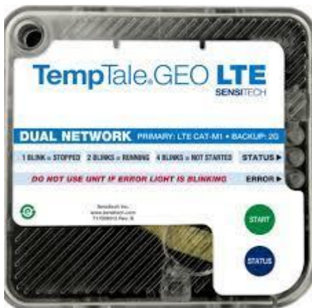
Figure 14 TempTale® GEO LTE (LxWxH = 115.5x121.5x25.5 mm., 207 gram) for detecting Temperature, Humidity, Light and location (Source: Sensitech)
