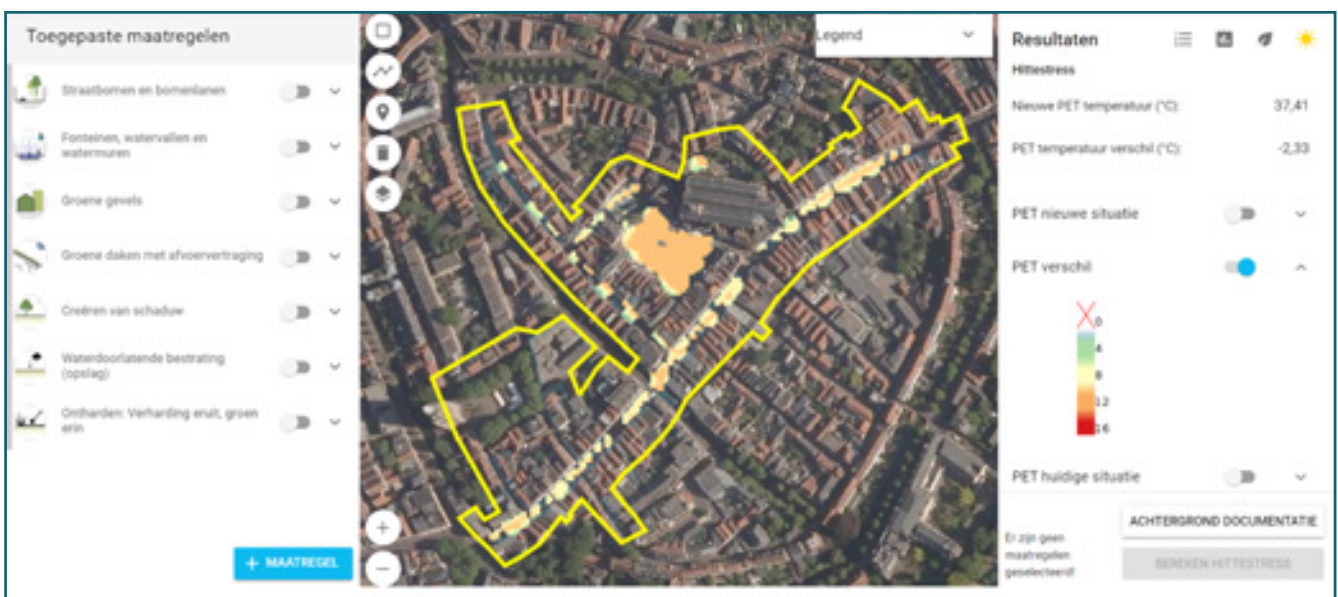
Figure 34: The PET difference between the situation without and with the site design implemented
