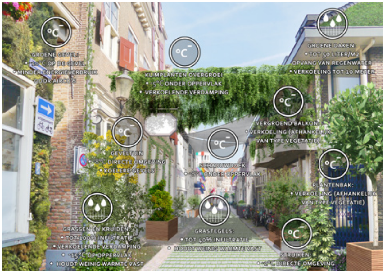
In the narrow street, smaller and flexible interventions are used, in comparison to the wide street. Climbing plants covers and shading covers provide shade. The planters are moveable. Façade gardens are applied in front of building facades.
