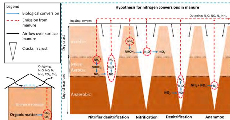
Figure 2. hypothesis of the nitrogen conversion pathways taking place in anaerobically stored manure as well as in the crust layer during storage.
