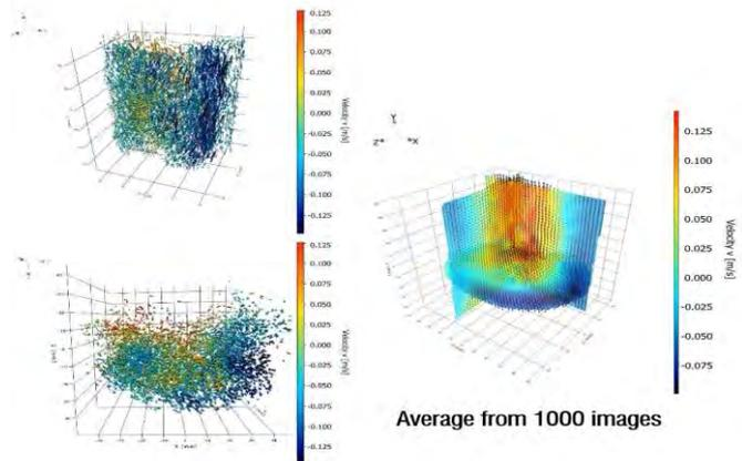
Figure 2 Time-resolved (left) and time-averaged (right) velocity distribution of liquid in the reactor
