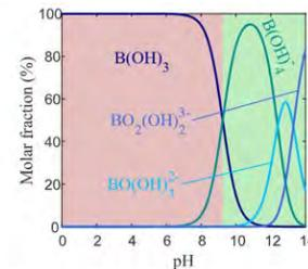
Figure 1 Speciation of boron as function of pH.
