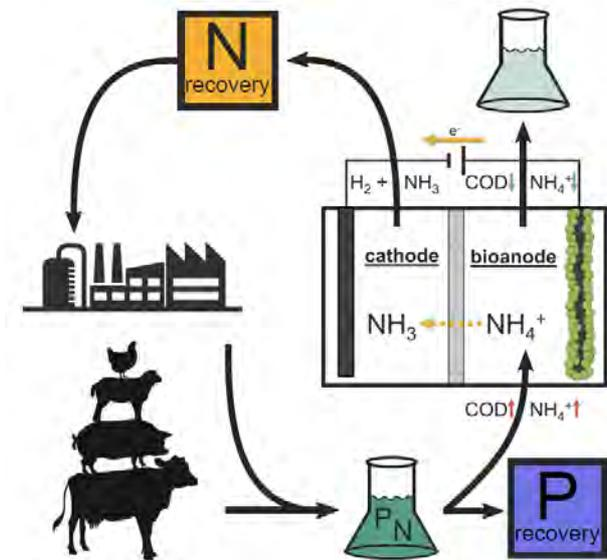
Figure 1: Nutrient removal and recovery cycle.
