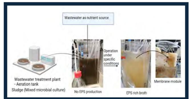
**Figure 2.** Changes of membrane bioreactor inoculated with aerobic mixed microbial culture during EPS production process. EPS production starts under specific process conditions (nitrogen limitation coupled with short solid retention times). During the production mixed liquor becomes viscous as a sign of presence of EPS.
