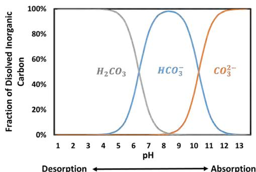
**Fig. 1.** Fraction of chemical species as function of the solution pH for the H<sub>2</sub>O-CO<sub>2</sub> system at 25 °C.
