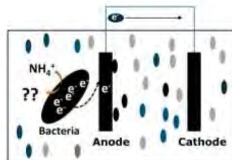
Figure 2 Concept of an anaerobic ammonium oxidation bioelectrochemical system integrating with electricity recovery.
