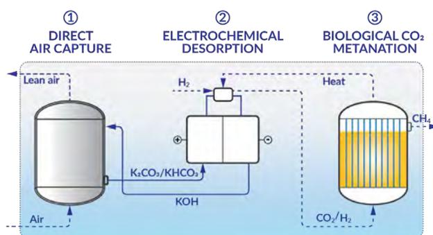
to keep methanogens at optimal metabolic activity. Finally, to reach efficient methane production, individual mass and energy flow need to be optimized in terms of energy requirements (kJ/mol CO<sub>2</sub>), and product yield (mol CH<sub>4</sub>/m<sup>3</sup> air).
