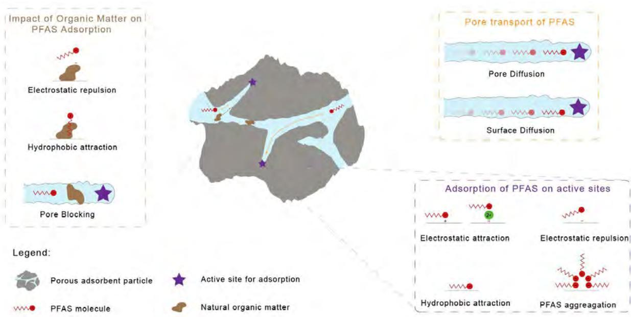
Figure 1. Mechanistic interactions between PFAS and adsorption material that will be studied
