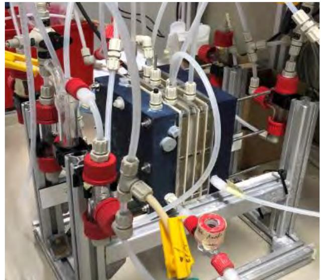
Figure 2: Microbial electrolysis cell removing ammonium from wastewater.
