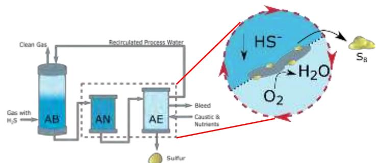
Fig. 1 - Schematic of the current biodesulfurization process and the shuttling capacity that occurs between the anaerobic (AN) and the aerobic (AE) reactors.
