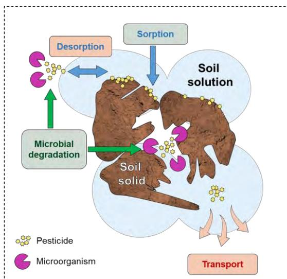
Figure 1. Schematic of processes governing pesticide fate in soil solution.
