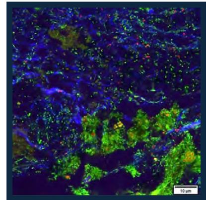
**Figure 1.** CLSM image of mixed liquor sample taken from EPS-producing bioreactor run under nitrogen limitation. The sample was stained with fluorescent dyes to show individual components of EPS; Sypro Orange (green, proteins), Calcofluor white (blue, polysaccharides), Syto 63 (red, DNA).
