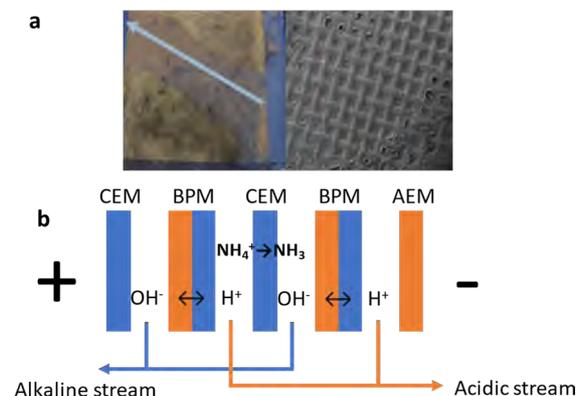
**Figure 1.** (left) Inorganic scaling of CEM in ES ammonia recovery. MEA: membrane electrode assembly, CEM: cation exchange membrane, ED: electrodialysis, LLMC: liquid-liquid membrane contactor. **Figure 2** (above) **a.** Inorganic scaling in CEM and spacers of ES. The arrow shows the direction of the flow. **b.** ES with possible production of acidic and alkaline streams. The possible use of these streams still needs investigation. AEM: anion exchange membrane, BPM: bipolar membrane.
