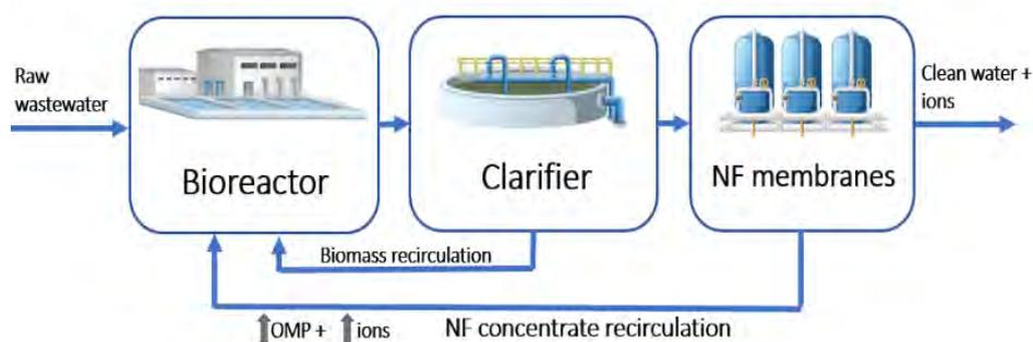
Figure 1 The proposed process, a combination of nanofiltration and biological treatment.
