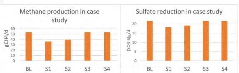
4 scenarios of heat recovery from domestic wastewater, from household (1) to different locations in sewers (2-4), are simulated in GIS to estimate the thermal energy and temperature dynamics. Together with a simplified sewer bioprocess model, the impact of heat recovery from wastewater on sewer gas formation can be estimated.
