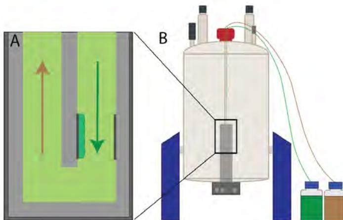
**Figure 2.** (Left) A schematic illustration of what the MR set-up might look like. (A) The biofilm reactor inside the MR sensor. (B) The MR scanner with the detector (gray), connected to influent (green) and effluent (brown) lines.
