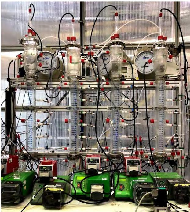
Figure 1 Lab-scale UASB reactors
