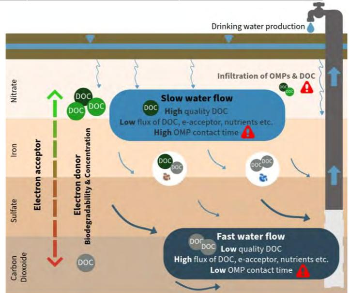
Figure 1 – Schematic representation of heterogeneity in aquifers, variability through DOC biodegradability and quantity, redox conditions and flow regimes foster microbial niches affecting biodegradation capacity.
