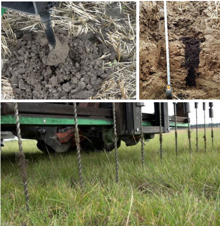
Figure 3. Top: Large borehole drill (left) with potting soil as stabilizing substrate(right). Bottom: Small borehole drills.
