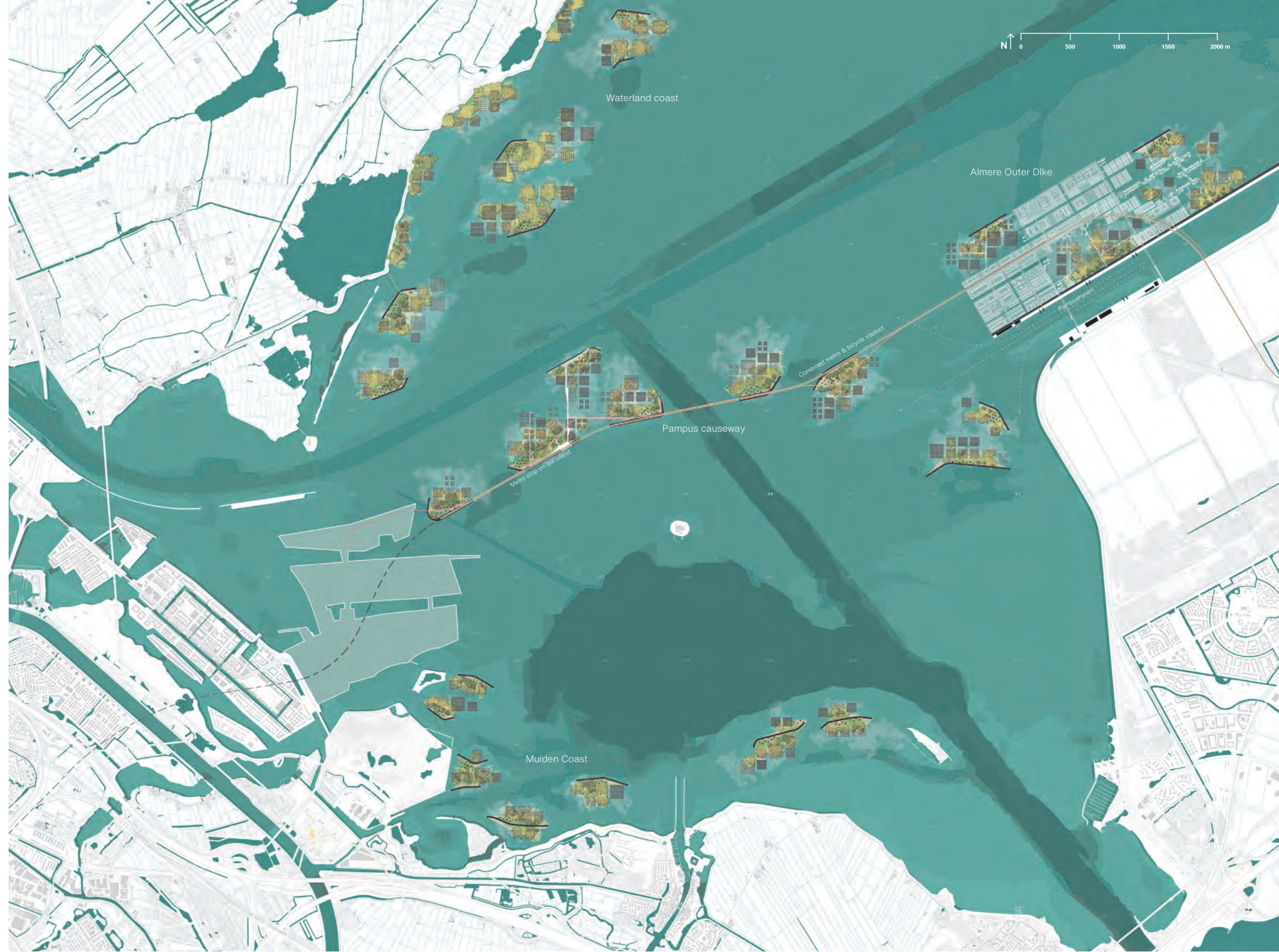
The modules combine into strings of islands and foreshores that slowly turn into land. Three strands of islands are envisioned: one along the Waterland coast, one along the Muiden coast and one right through the middle. The middle strand provides a base for a rail infrastructure causeway and viaduct, as well as an island for recreation and guiding principles for a new urban expansion of Almere.
